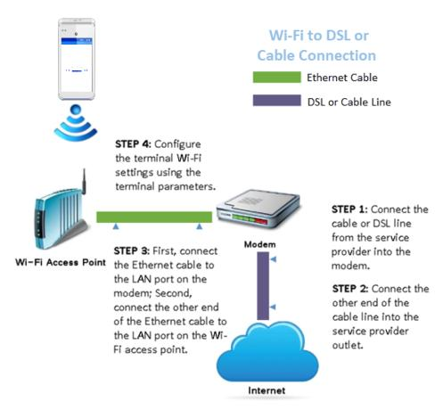
The A920 supports Wi-Fi for network and internet access. Wi-Fi is a wireless computer network that links two or more devices using wireless communication to a local area network (LAN) within a limited area, such as store or office building.
